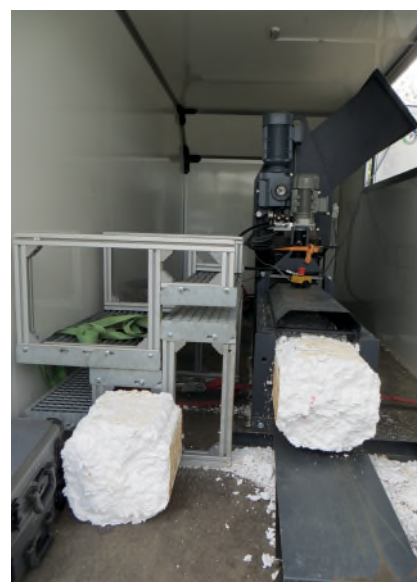
Figure 19 To significantly reduce the volume of insulation waste for transportation and storage before recycling treatments, mobile units to be used at demolition sites have been developed. ©Ralf Pasker
